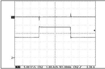
Figure 5: Output voltage response to step-change in load current (50 % -75 %-50 % of Iout(max);  $dI/dt = 0.2 A/\mu s$ ). Load cap: 1  $\mu F$  ceramic capacitor. Ch 1: Vout, Ch 2: Iout. Timescale: 1.00ms/div.
