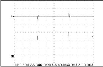
Figure 5: Output voltage response to step-change in load current (50 % -75 %-50 % of Iout(max);  $dI/dt = 0.2 A/\mu s$ ). Load cap: 1  $\mu F$  ceramic and 15  $\mu F$ tantalum capacitors. Ch 1: Vout, Ch 2: Iout. Timescale: 1.00ms/div.
