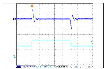
Figure 6: Output voltage response to step-change in input voltage (1000 V/ms). Load cap: 1 µF ceramic capacitor. Ch 1: Vout, Ch 2: Vin. Timescale: 1.00ms/div.
