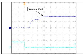
Common Figure 1: Typical startup waveform. Input voltage pre-applied, ON/ OFF Pin on Ch 2. Output voltage normalized. Timebase: 4msec/div.
