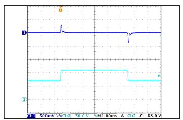
Figure 6: Output voltage response to step-change in input voltage (1000 V/ms). Load cap:  $1 \mu F$  ceramic and  $15 \mu F$  tantalum capacitors. Ch 1: Vout, Ch 2: Vin. Timescale: 1.00 ms/div.
