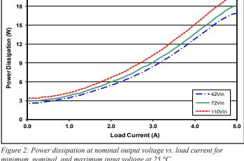
minimum, nominal, and maximum input voltage at 25 °C.
