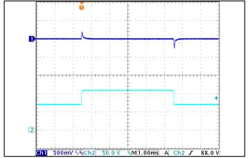
Figure 6: Output voltage response to step-change in input voltage (1000 V/ms). Load cap:  $1 \mu F$  ceramic and  $15 \mu F$  tantalum capacitors. Ch 1: Vout, Ch 2: Vin. Timescale: 1.00 ms/div.
