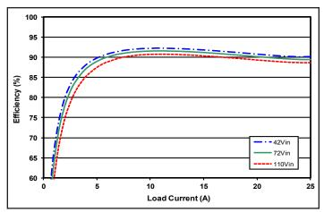
Figure 1: Efficiency at nominal output voltage vs. load current for minimum, nominal, and maximum input voltage at 25c°C.
