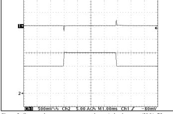
Figure 5: Output voltage response to step-change in load current (50 % -75 % -50 % of Iout(max); dI/dt = 0.2  $A/\mu s$ ). Load cap:  $I \mu F$  ceramic and  $I5 \mu F$  tantalum capacitors. Ch 1: Vout, Ch 2: Iout. Timescale: I.00ms/div.
