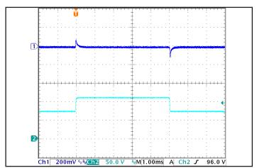
Figure 6: Output voltage response to step-change in input voltage (1000 V/ms). Load cap: 1 µF ceramic and 15 µF tantalum capacitors. Ch 1: Vout, Ch 2: Vin. Timescale: 1.00ms/div.
