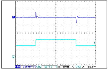
Figure 6: Output voltage response to step-change in input voltage (1000 V/ms). Load cap: 1 µF ceramic and 15 µF tantalum capacitors. Ch 1: Vout, Ch 2: Vin. Timescale: 1.00ms/div.
