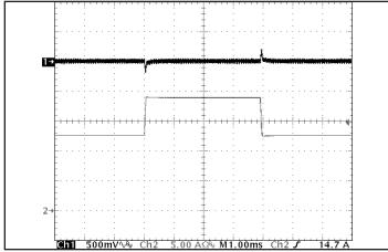
Figure 5: Output voltage response to step-change in load current (50 % -75 % -50% of lout(max);  $dI/dt = 0.2 \ A/\mu s$ ). Load cap:  $1 \ \mu F$  ceramic and  $15 \ \mu F$  tantalum capacitors. Ch 1: Vout, Ch 2: Iout. Timescale: 1.00 ms/div.
